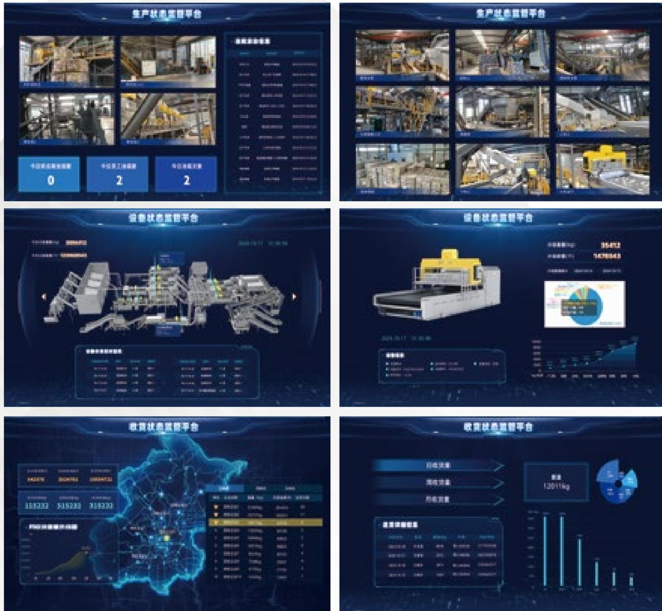
The system includes smart weighing, impurity deduction and settlement features. Tracks delivery vehicle/driver info, recycling station location
